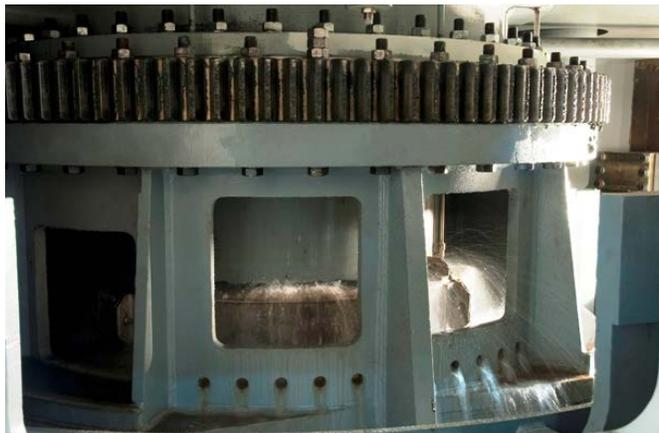
Water cooling system keeps the HD cool to ensure reliable operation.
