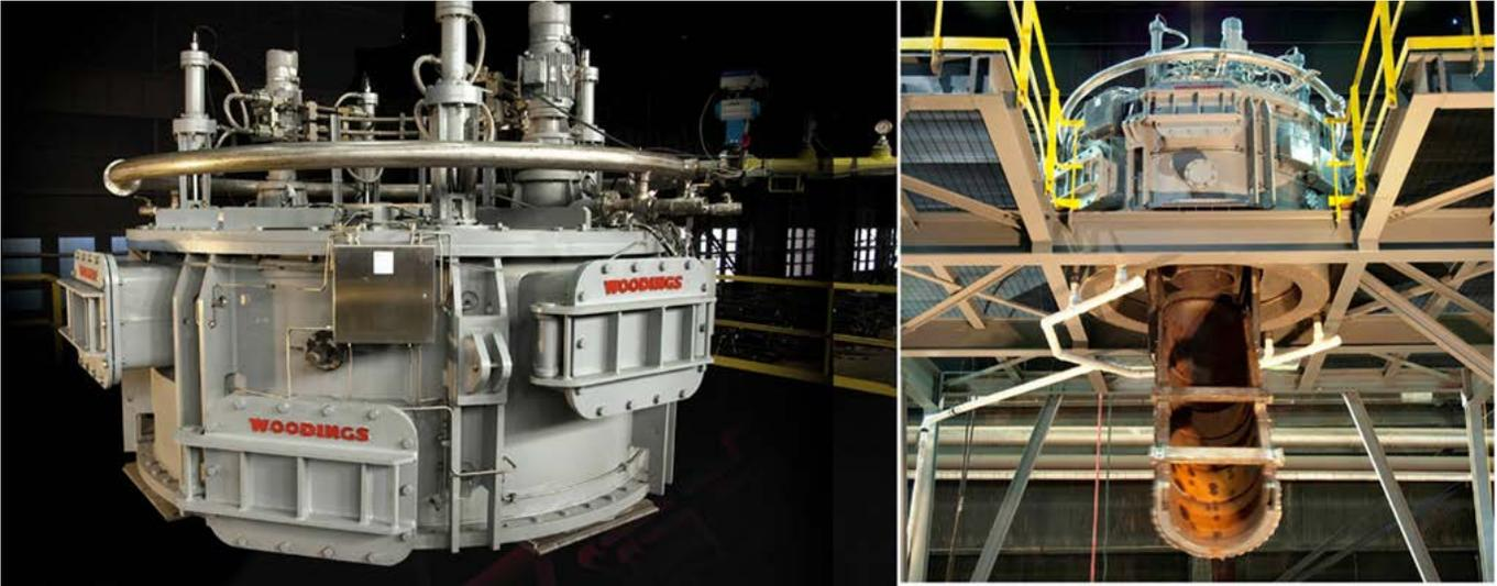
*Hydraulic cylinders replace the traditional mechanical function for tilting the revolving chute.*
