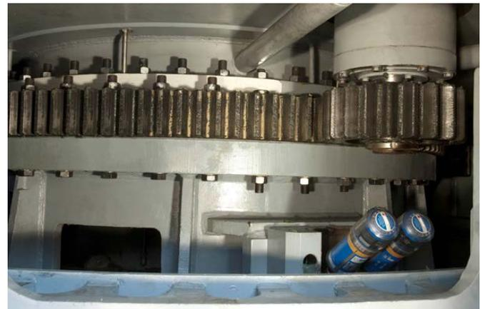
Rotation of the chute is accomplished with a simple gearbox and electric motor.
